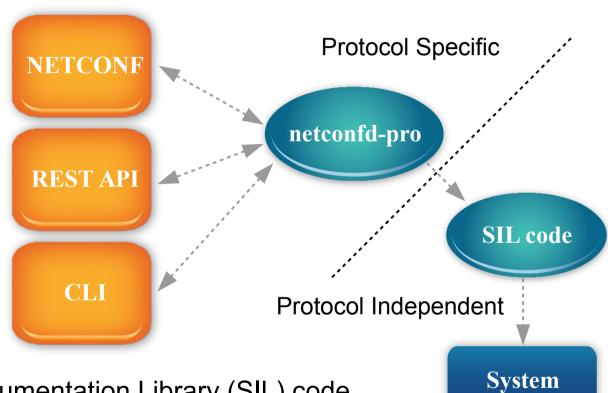
Server Instrumentation Library (SIL) code is protocol-independent so engineers can focus on managing the system, not all the management protocols
