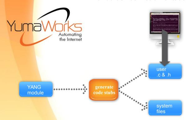
The user and system code is then built into a dynamically loadable library – a SIL (Server Instrumentation Library) and for distributed Systems a SIL-SA (SIL-Sub Agent).
