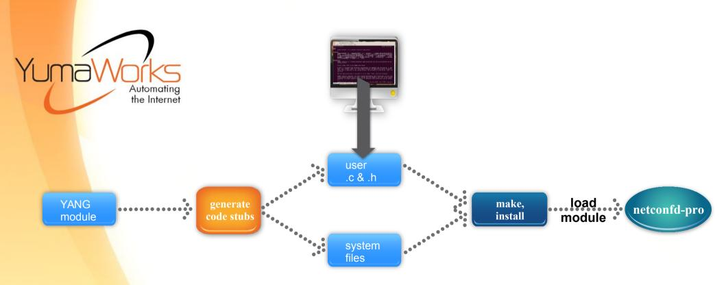
Bundles can group collections of YANG modules together into a dynamic library that can be loaded with one command.
